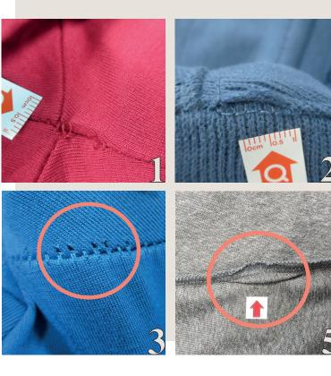
**Broken or skipped stitches:** when the sewing thread breaks or when one or several stitches are skipped.
